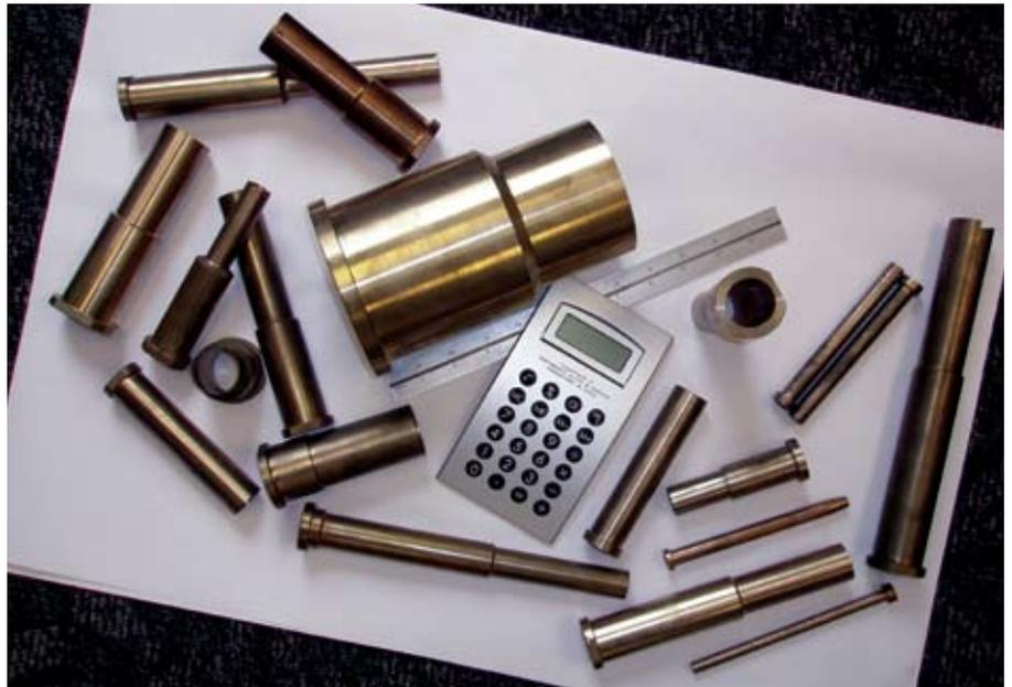
An assortment of custom made sleeves using aluminum bronze alloy ranging to fit inner cores from under .250" up to over 3", typically with wall thickness of not less than .030" per side.
