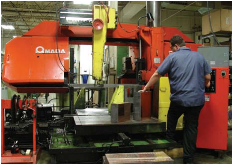
Sawing of 5-inch thick 30 Rockwell "C" copper alloy plate with carbide tipped saw blade.
